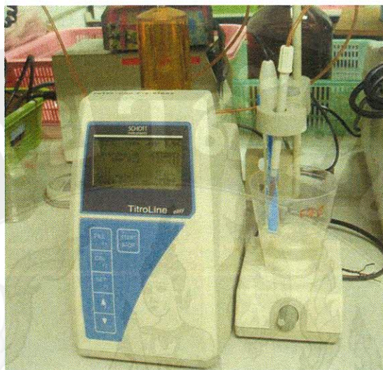
Figure 16 Titratable acidity determined by using autotitrator
