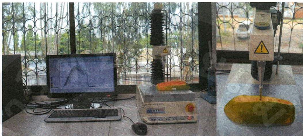
Figure 11 Papaya fruit firmness measuring by texture analyzer
