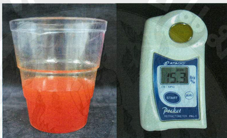
Figure 15 Total soluble solids content of papaya fruit juice measuring by digital refractometer
