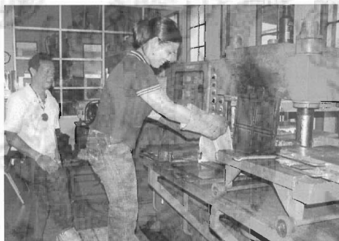
Figure D4. Vulcanizing or curing the compound rubber using a hydraulic press.
